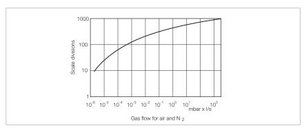
Variable leak characteristic for the variable leak valve with isolation valve
