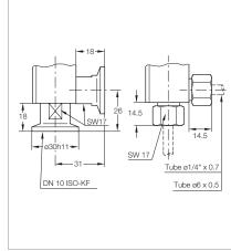
Connection dimensions for small valves micro
