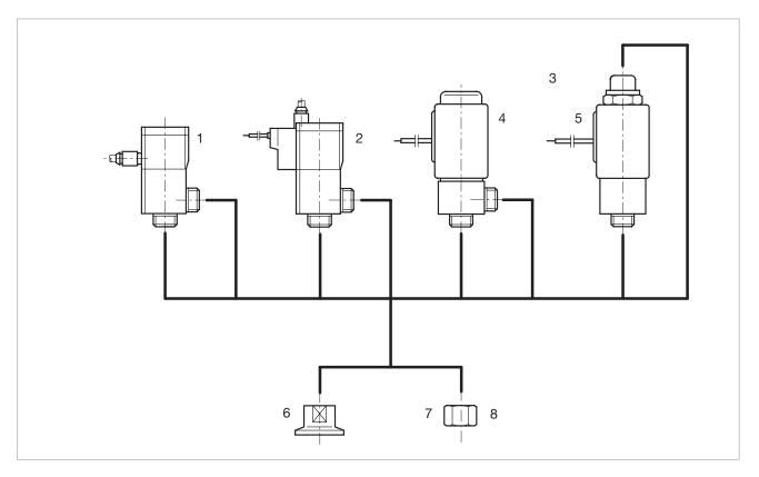
Leybold small valves **micro** are available with any of three drive systems, two types of body and three adaptors.
