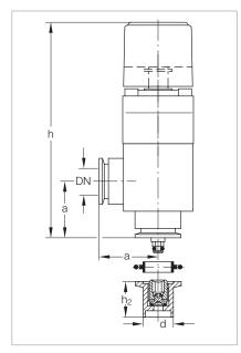
Dimensional drawing for the sealing valves
