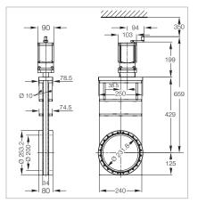
Dimensional drawing for the UHV gate valve DN 200 CF
