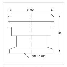
Dimensional drawing for the pressure relief valve
