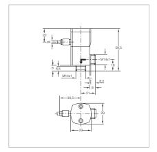
Dimensional drawing for the pneumatically actuated small valves **micro**
