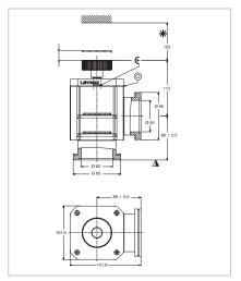
Dimensional drawing for the right-angle valves, bellows-sealed, manually operated, dimensions in mm
