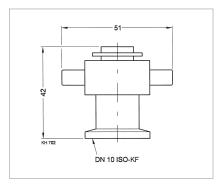
Venting valves are used to vent small vacuum systems.
