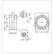
Connection dimension for CF flanges DN 63 CF to DN 160 CF
