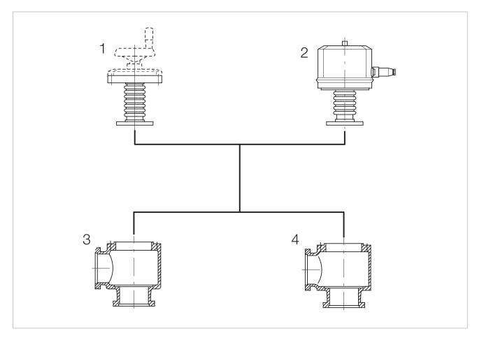
Leybold valves with ISO-K flanges are available with any of two drives and either of two bodies.
