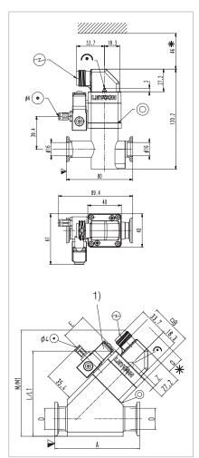
Dimensional drawing for the straight-through valves with fitted pilot valve (EP) without pilot valve (P) (on top DN 16 ISO-KF, stainless steel)
