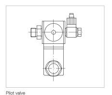
A range of pilot valves is available for actuation of the electropneumatic ISO-KF valves, which cover all commonly used control voltages.
