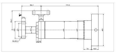
Dimensional drawing for the all-metal variable leak valves
