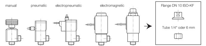
Micro valves overview (right-angle / straight-through valves) Example dimensions for electromagnetic straight-through valve: 2 x 10 KF, approx. 100 mm long Adaptors for micro valves
